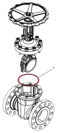
There is a sealing element (Fig. 9/1) between the body and the body cover to prevent the pipeline medium from escaping from the body. If leaks occur, the sealing element can be replaced by employees of the operating company ( & *Chapter 8.3.2 'Replacing the gland packing and cover gasket' on page 73*).
