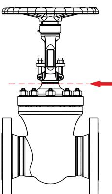
Fig. 16: Upper edge of the insulation
