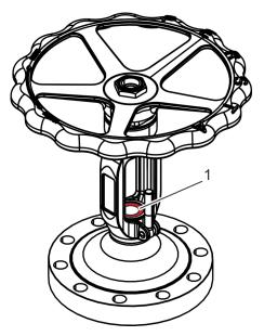
Fig. 23: Removing the gland packing
