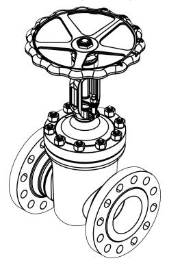
The stem is driven manually with the handwheel.
