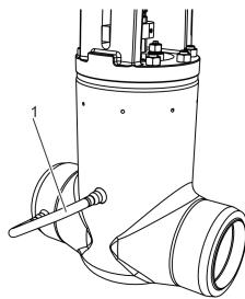
An equalizing pipe (Fig. 5/1) is used to create a connection between the 3rd chamber (Fig. 2/3) and the pressurised side (Fig. 2/1 (1st chamber)) of the valve.
