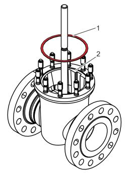
**8.** Remove the gasket (Fig. 24/1) from the groove (Fig. 24/2) in the body.
