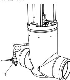
A safety valve (Fig. 6/1) attached to the nozzle (Fig. 3/2) discharges critical pressures.
