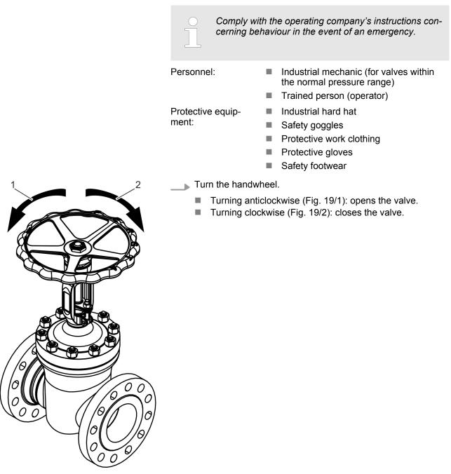
*Fig. 19: Manual actuator: Operating the handwheel in an emergency*
