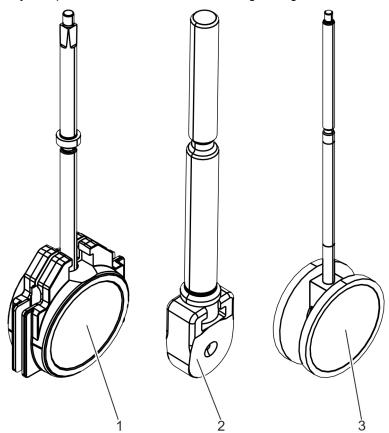
Fig. 10: Versions of the shut-off element
