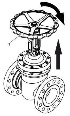
Fig. 22: Turning the handwheel
