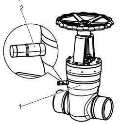
Fig. 15: Closed nozzle on the body
