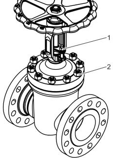
Fig. 21: Undoing the threaded connections
