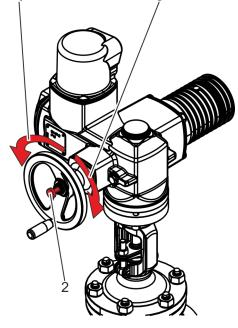
*Fig. 20: Electric actuator: Operating the handwheel in an emergency*
