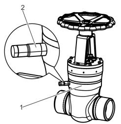
Depending on the application, the valve (Fig. 3/1) may need to be equipped with an external overpressure safety device by the operating company. In this regard, the valve can be delivered with a factory-sealed nozzle by the manufacturer (Fig. 3/2). The nozzle creates a connection from the outside to the 3rd Chamber (Fig. 2/3). External overpressure safety devices can be attached to the nozzle (Fig. 3/2).
