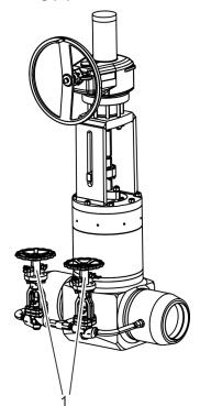
Fig. 4: Bypass with equalizing pipe (shown here: DSK 25 50–600)
