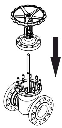
*Fig. 26: Attaching the cover and gland follower flange*
